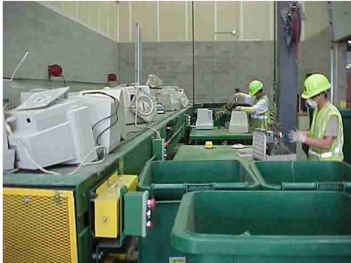
Line showing 2 Demanufacturing Work Stations
